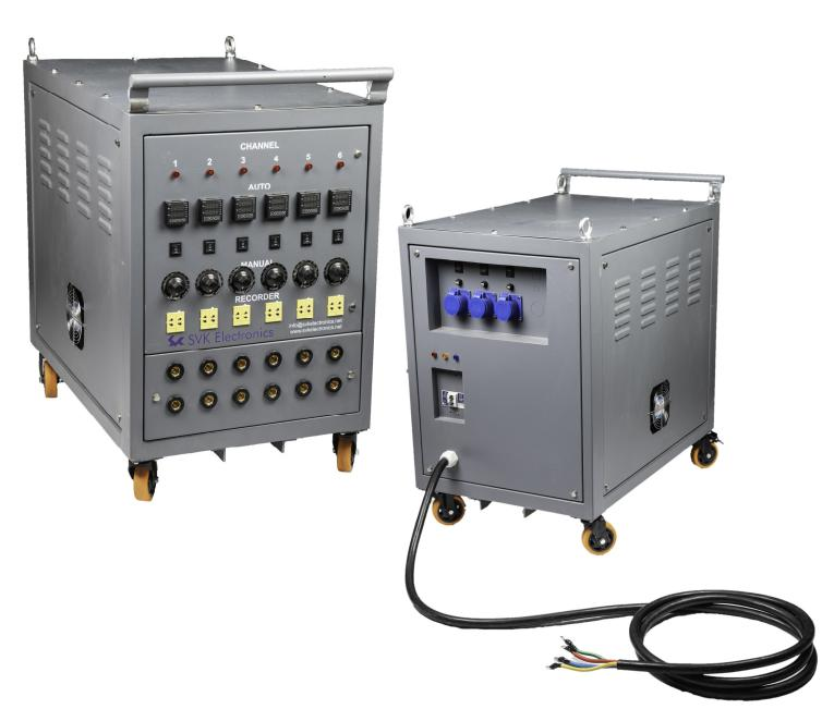
The 75 kVA heat treatment unit has been robustly constructed to provide power to electrical resistance heaters at 60 volts, suitable for site and shop working. It is specifically designed for localized Pre and Post Weld Heat Treatment using Electrical Resistance
